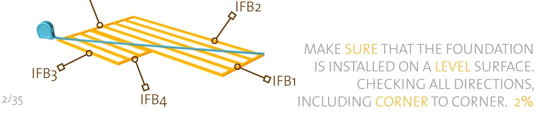
ATTACH FOUNDATION BEAMS WITH SCREWS.
