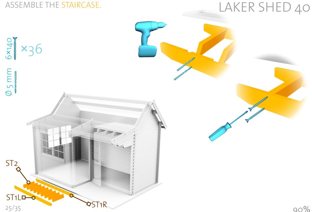
SET THE **STAIRCASE** AT THE RIGHT SPOT, ATTACH THE FIRST **HALF** OF THE LADDER **FITTINGS** TO THE WALL **WITH** SCREWS.
