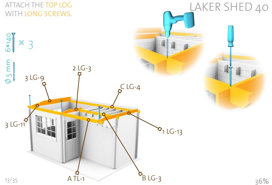
INSTALL THE GABLES WITH LONG SCREWS TO THE WALL LOGS ON THE FRONT AND REAR WALLS.
