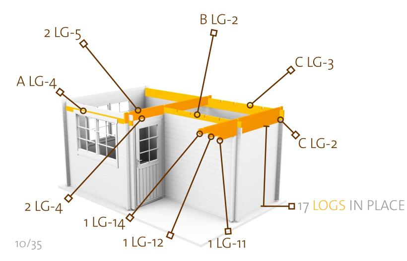
INSTALL THE CEILING BEAMS AND ATTACH THEM WITH SCREWS.
